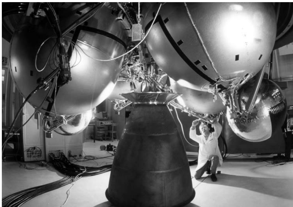
Figure 3.9. The Aestus engine on Ariane 5. The high-expansion ratio nozzle and two of the four propellant tanks can be seen. Upper-stage engines should be short to reduce the overall length of the vehicle; here the propellant tanks cluster round the engine. Courtesy ESA.
