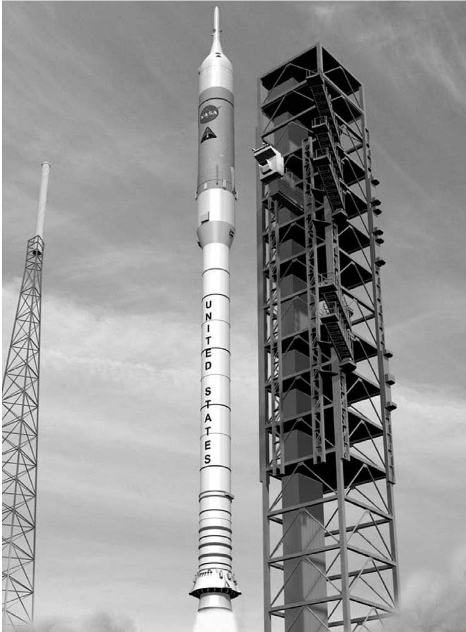
Figure 9.15. Artist's impression of an Ares I launch with crew onboard. The first stage is a five-segment SRB and the second stage is powered by the J-2X engine and burns liquid hydrogen and liquid oxygen. The main engine of the Orion spacecraft performs the final orbital injection. Courtesy NASA.
