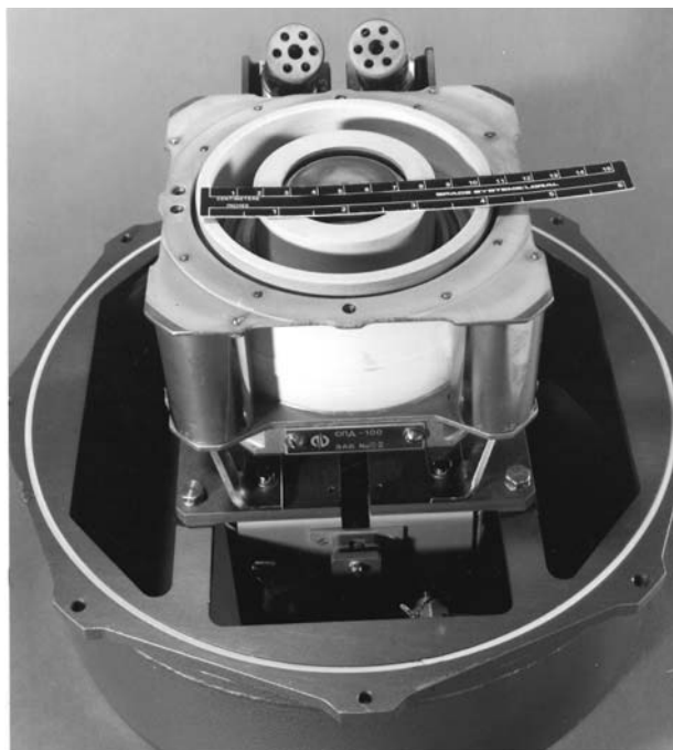
Figure 6.17. The Russian SP-100 Hall effect thruster. 100 mm diameter of the insulated cavity is shown by a ruler. The twin electron guns can be seen as well as two of the four coils that power the outer ring magnet. This is an SPT rather than a TAL device, it has a deep discharge cavity, insulated with boron nitride. Courtesy NASA.
