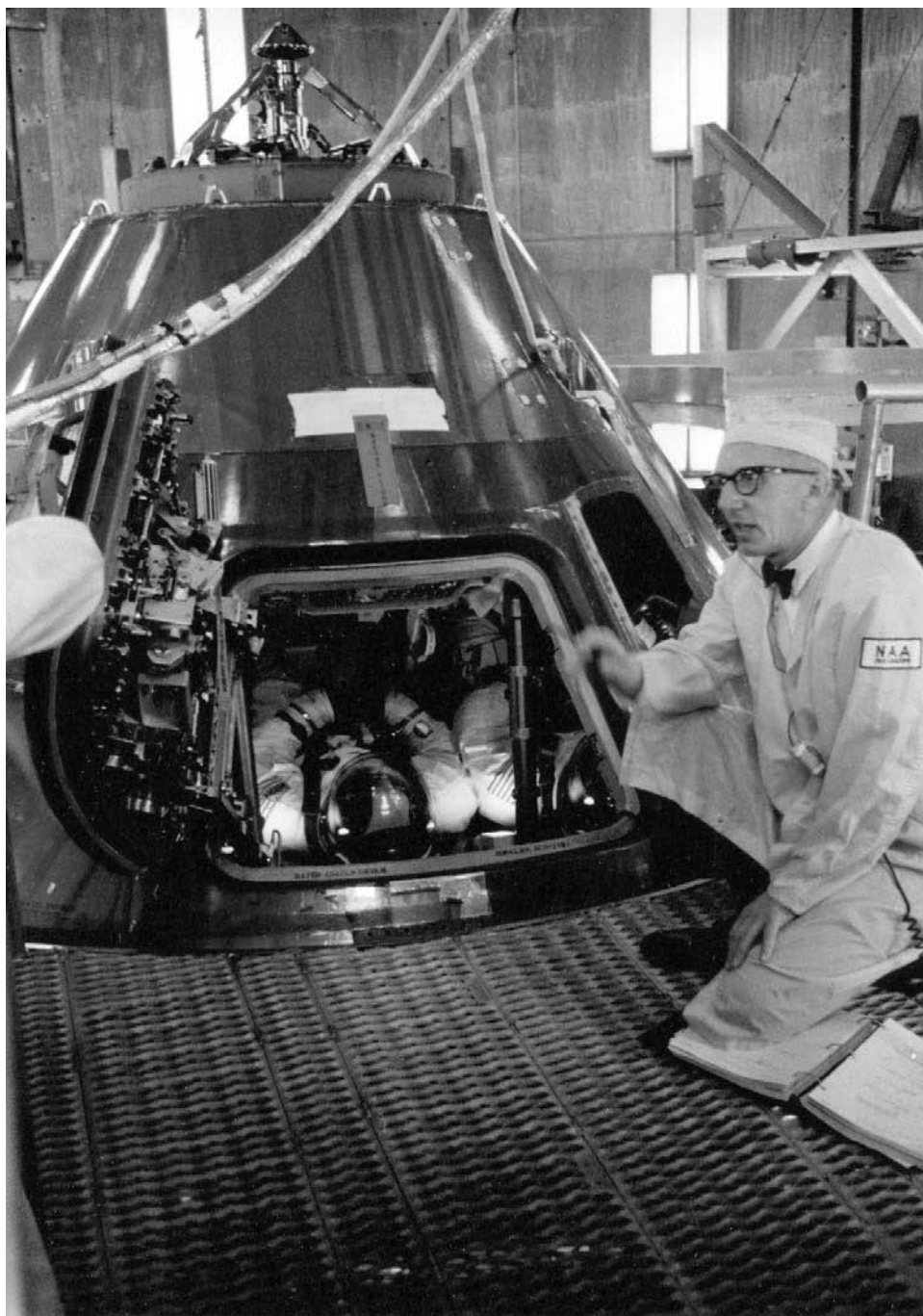
Figure 9.1. The Apollo Command Module inside the vacuum chamber, being prepared for space simulation tests. Courtesy NASA.
