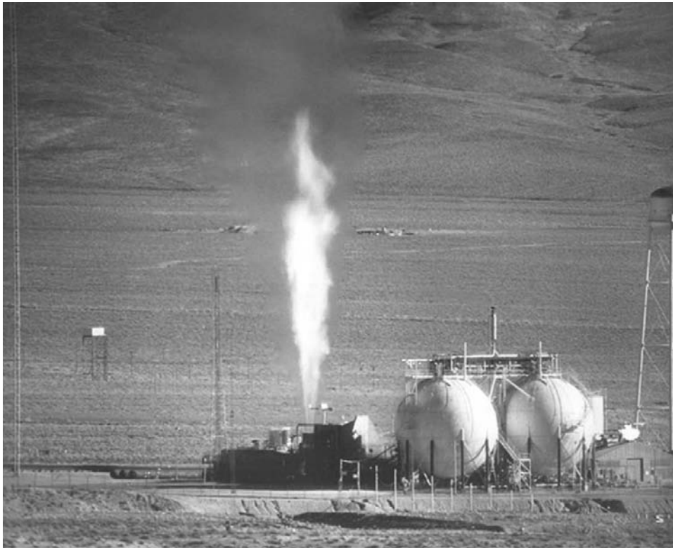
Figure 7.1. Actual test of a nuclear rocket engine at Jackass Flats in Nevada, as part of the NASA NERVA programme. The engine is firing vertically upwards, the storage tanks are for the liquid hydrogen. Courtesy NASA.
