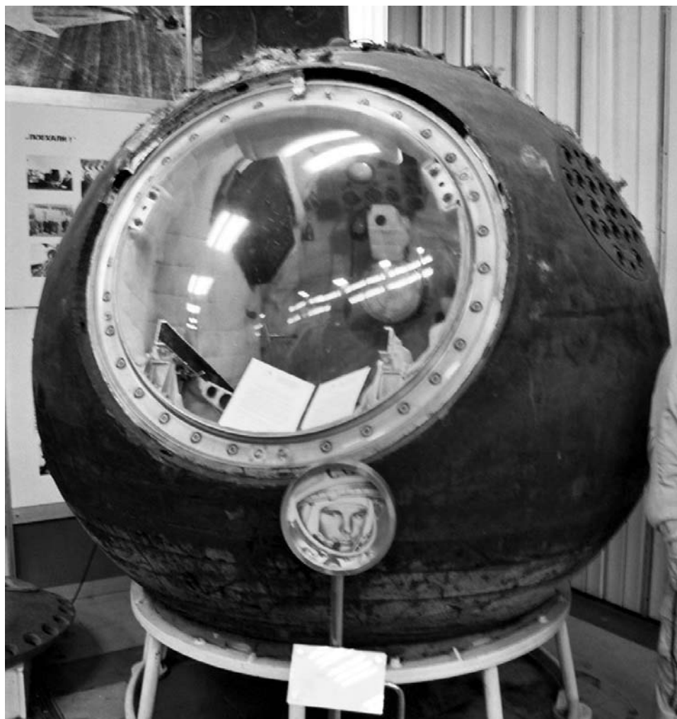
Figure 9.6. The Vostok capsule after landing; remnants of the thermal protection material are still attached. Courtesy RKK Energia.
