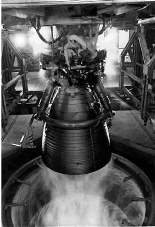
Figure 3.12. The Vulcain 2 under test. This is the new version of the Vulcain specified for Ariane 5. It uses a more oxygen-rich mixture to improve the mass ratio, and a longer nozzle to restore the exhaust velocity. Courtesy ESA.
