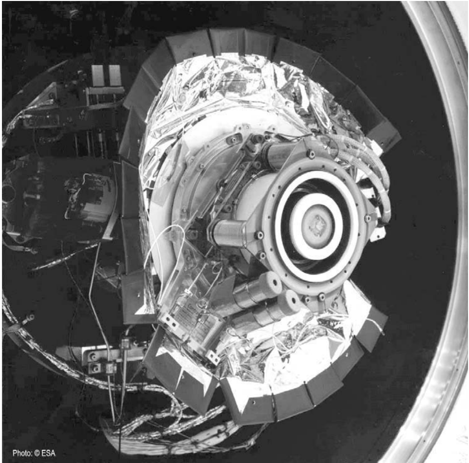
Figure 6.28. The PPS 1350 Hall thruster mounted on SMART-1. This device has operated faultlessly in space for over a year now as SMART-1 is lifted to the Moon's orbit. Courtesy ESA.
